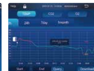
Real-time display of operation data real-time display of temperature, CO 2 concentration and O 2 concentration, and the data during the culture cycle can be viewed at any time
